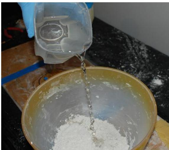
When I measure out the dry I try to imagine the amount it would take to cover my positive to a thickness of  $\frac{1}{2}$  inches. I then add cold water slowly to the dry mix stirring with a whisk till I get a mixture of even consistency about as thick as a milkshake.
