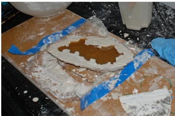
Pre-fire your mold to 50 degrees Fahrenheit above your glass forming temp. Once fired the mold can be carved and cleaned. (do not use water) It is important to eliminate any undercuts. Spray with isopropyl alcohol and kiln wash till you have a light coating. Then fill with glass and fire.
