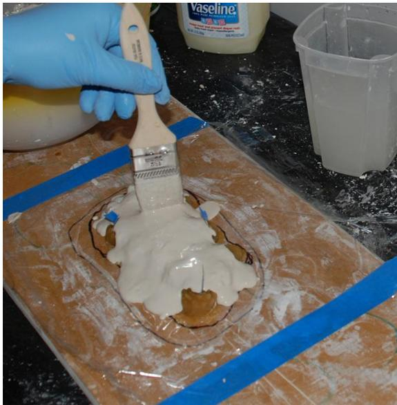
Once the mixture is the right consistency pour some on the positive then brush it into the surface of the piece. This pushes the mold mixture into the details and pops air bubbles on the surface.
