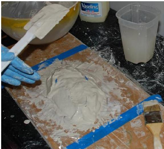
It is important that you don't make too little Castalot. If your Castalot fully sets and you add more because of a thin spot, the patch may delaminate from the main mold after pre-firing. It is important to determine early on whether you will need more material to cover your positive.
